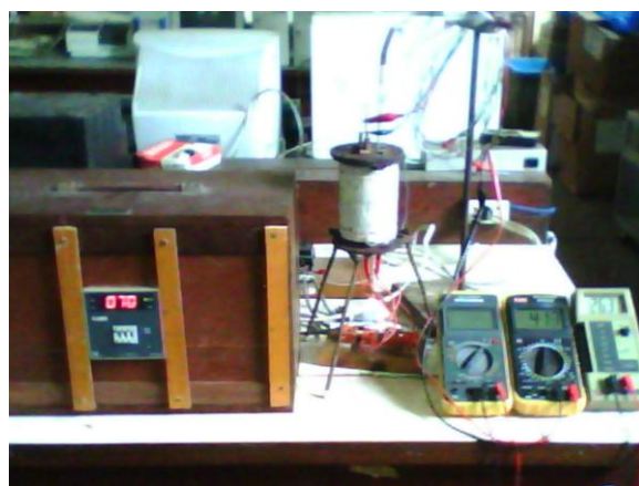
Fig 2 Experimental setup of temperature dependent electrical conductivity measurement
